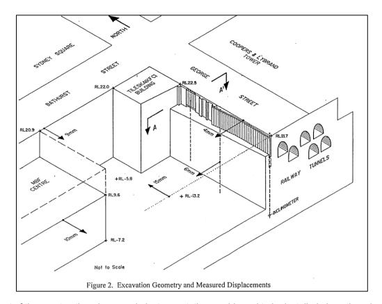
As part of the construction phase work, instrumentation would need to be installed along the edge of the basement footprint and possibly within the nearby tunnels to monitor progress of the works. Such monitoring may include inclinometers, tunnel survey, tunnel convergence monitoring, vibration monitoring and surface survey monitoring.
